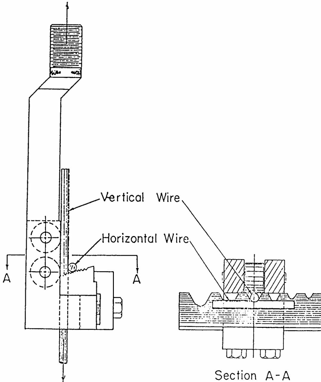
Note 3 - See specification A 185 for additional information on weld shear testing. A detailed drawing showing complete dimensions of testing fixture may be obtained from ASTM by order Adjunct No. 12-101850-00.
